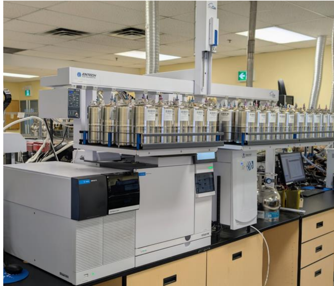
Agilent 7010D GC-MS/MS Entech 7200-PFAS pre-concentrator and SK-75 autosampler
